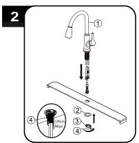
Place faucet (1) through the hole in the countertop. Secure the faucet (1) to the countertop using the metal washer (2), and mounting nut (3) provided. Tighten screws (4) with a phillips screwdriver. Do not overtighten.
