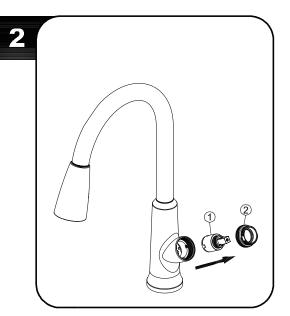
Loosen the cap (2) by turning it counter-clockwise and lift out the cartridge (1). Insert new cartridge. Reinstall the handle.
