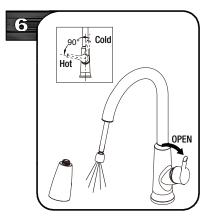
After the installation is complete, pull the hose assembly out of the spout and remove the spray head by unscrewing it from the hose in a counterclockwise direction. Turn on the water supply to flush debris from the faucet. Run the hot and cold water for at least one minute each. Important: This flushes away any debris
