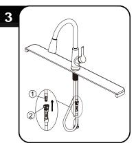
Push the quick connector (2) firmly upward and attach it to the receiving block (1). Pull down moderately to ensure the connection has been made.
