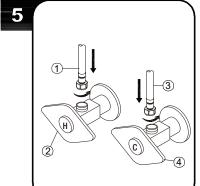
Thread the nut (1) on the hot water supply line onto the outlet of the hot water supply valve (2) and tighten with wrench. Do not overtighten. Thread the nut (3) on the cold water supply line onto the outlet of the cold water supply valve (4) and tighten with wrench. Do not overtighten.
