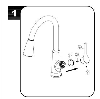
Shut off water supply. Unscrew the set screw (4) on the handle (3). Remove the handle (3) and loosen the screw (2) from valve stem. Loosen the cap (1).
