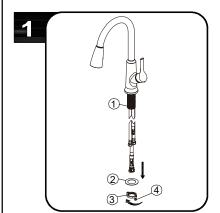
Before installation, shut off water supplies, remove old faucet. Next, remove metal washer (2) , nut (3) and screws (4) from shank (1).
