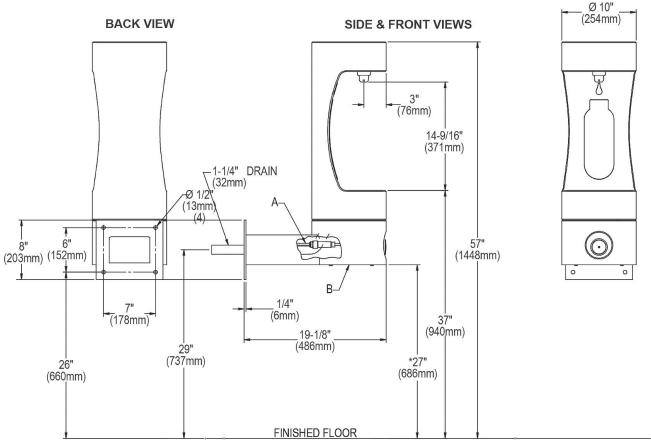
$\underline{A} = 3/8$ " O.D. Unplated copper tube connect. Shut off valve by others.
