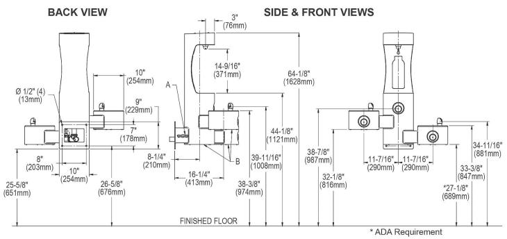
A = 3/8" O.D. UNPLATED COPPER TUBE CONNECT - SHUT OFF VALVE BY OTHERS
