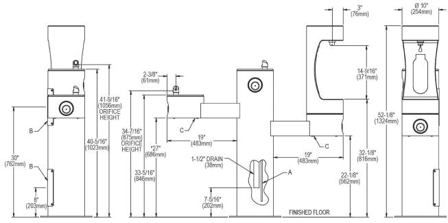
A = 3/8" O.D. Unplated copper tube connect. Shut off valve by others. B = Access panel( $8" \times 10"$ ).
