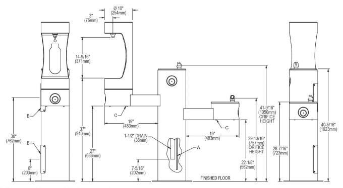
A = 3/8" O.D. Unplated copper tube connect. Shut off valve by others. B =  $Access panel(8" \times 10")$ .
