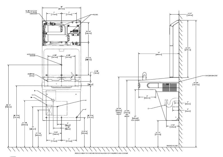
LEGBND: = Recommended Water Supply location. Shul-off Valve (not funished) to accept 3/8° O.D. unplated copper tube. Up to 3° (76mm) maximum out from wall. = Recommended Water Outlet location. To accommodate 1-1/4° nominal drain. Drain shub 2° (51mm) out from wall. D = Bertinda Supply (3) Wire Received Duplex Outlet. = Insure proper vehilation by markinging 4° (15mm) minimum clearance from cabinet louvers to wall. Note: New Installations Mat Up Grown Gault Claudit Interupter (GRCI).
