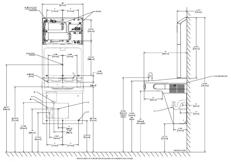
r Supply location. Shut-off Valve (not furnished) to accept 3/8" O.D. unplated copper tube. Up to 3" (76mm) maximum out from wall. • Outlet location. To accommodate 1-1/4" nominal drain. Drain stub 2" (51mm) out from wall.
