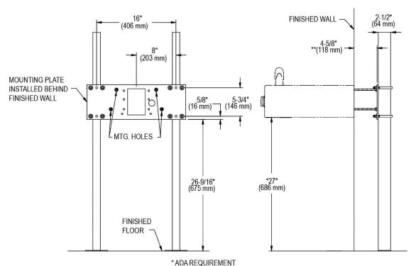
\*\* WITH STANDARD STUD LENGTH OF 6 INCHES NOTE - AFTER INSTALLATION, U-BOLTS AND THREADED RODS MAY NEED TO BE TRIMMED.
