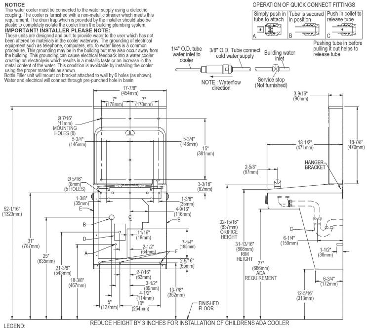
A = Recommended Water Supply location. Shut-off Valve (not furnished) to accept 3/8" O.D. unplated copper tube. Up to 3" (76mm) maximum out from wall. B = Recommended Waste Outlet location. To accommodate 1-1/4" nominal drain. Drain stub 2" (51mm) out from wall.
