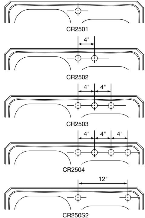
ALL DIMENSIONS IN INCHES, TO CONVERT TO MILLIMETERS MULTIPLY BY 25.4.
