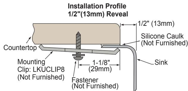
Designed to affix to the underside of any solid surface countertop.
