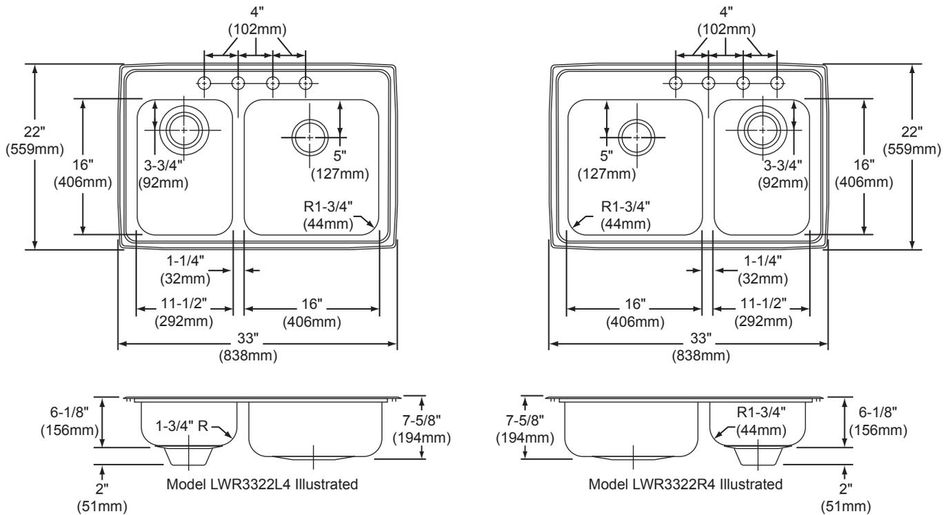
**Hole Drilling Configurations**
