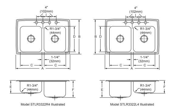
Hole Drilling Configurations 1-1/4" (32mm) Diameter Faucet Holes on 4" (102mm) Centers
