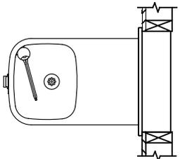
USE THESE DIMENSIONS WITH HAWS MODEL: 1109, 1109.14, 1109FR, 1109FRB, 1109FRP AT 22-1/4" HEIGHT TO ACHIEVE 30" MAX. CHILD ADA BUBBLER HEIGHT \* NOTE: MUST USE PARALLEL APPROACH WITH THIS BOWL COMBINATION.
