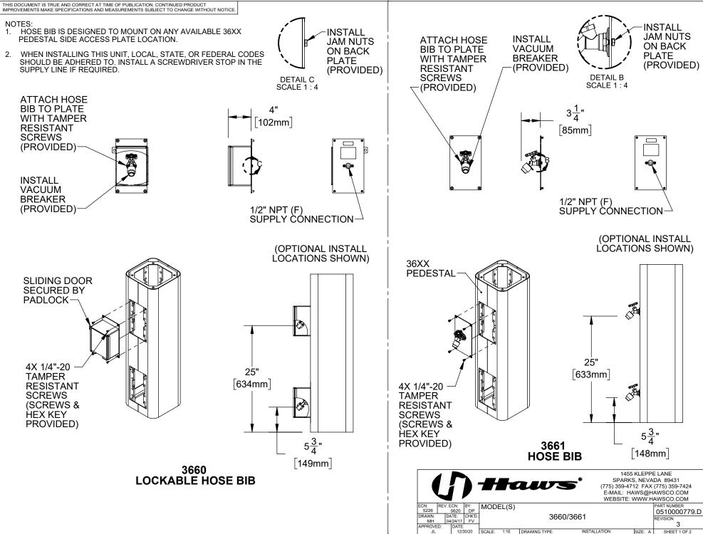
**CAUTION!** THIS HOSE BIB ACCESSORY IS NOT FREEZE RESISTANT! TO PREVENT DAMAGE TO THE UNIT AND A POTENTIAL FLOODING HAZARD, DO NOT INSTALL IN LOCATIONS THAT HAVE THE POTENTIAL TO FREEZE.
