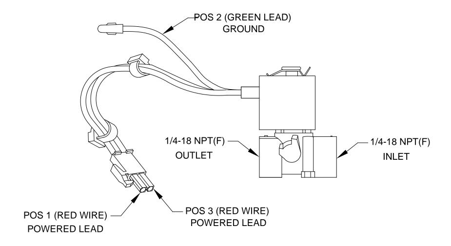
MUST BE USED IN CONJUNCTION WITH 24VAC TRANSFORMER AND SENSOR.
