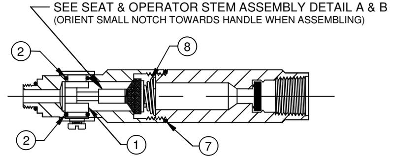
CLEAN VALVE THOROUGHLY AND LUBRICATE 'O' RINGS WITH 'O' RING LUBE BEFORE REASSEMBLING.
